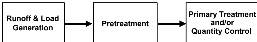
Figure 3.1.6-1 Generalized Stormwater Treatment Train
